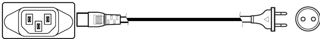
Use the included cable only. Connect one side to the DAC and then plug the other side into the wall outlet.
