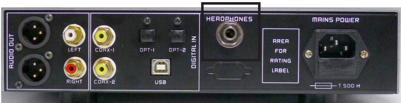
Instead of an amplifier and speakers, headphones can be used to listen to music. The headphones connector is located on the back side.
